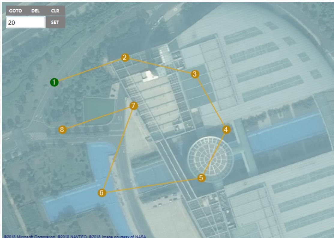
The map on the right side of the "SWARM" tab is used to perform path planning flight for a single drone. For the list of nodes on the left side, please select a single drone.
