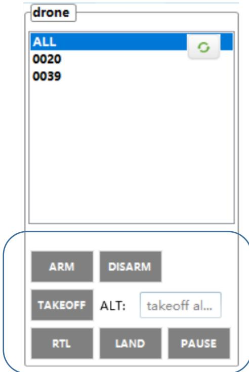
Select single or all online drones (ALL) to control the drone's simple operations such as unlocking, taking off, landing, and locking.
