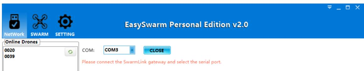
After connecting the SwarmLink gateway to the PC with the serial port tool, the software will automatically identify the serial port number of the serial device that has been connected.
