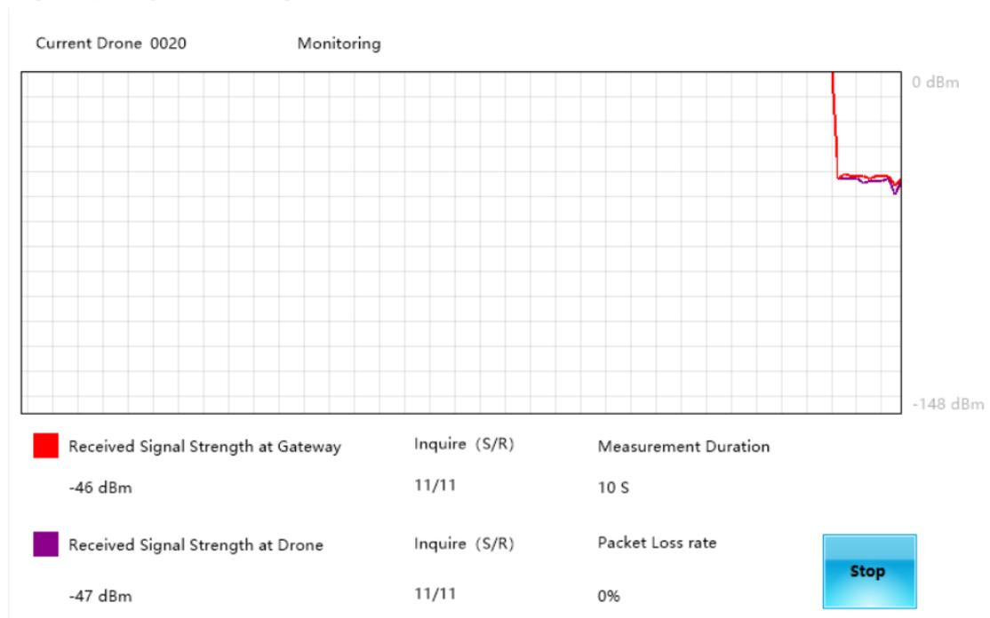
In the "Online drones" list, select a node and click the "Start Measurement" button to monitor the signal quality of the networking node.
