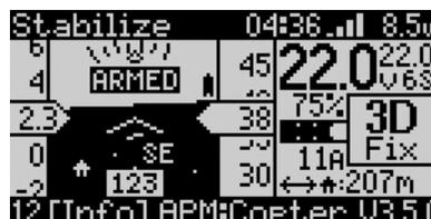
By validating [ENT], some of the information is replaced by the lowest cell voltage from the cell sensors (if used) or averaged from pack voltage along with the lowest recorded cell voltage, power draw from power modules (if used), and number of satellites and GPS fix quality (HDOP).
